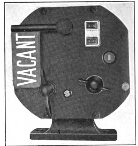
Fig. 3—Rear View of Taxameter showing half-mile travel
